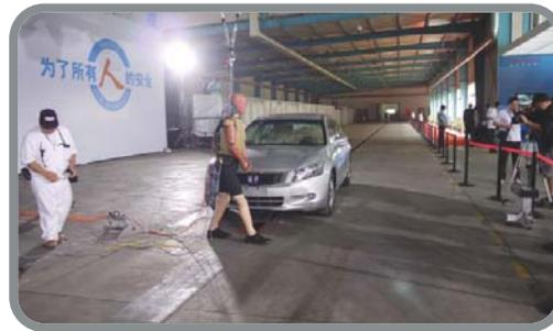
CATARC using Honda POLAR for Pedestrian Dummy Crash Test
