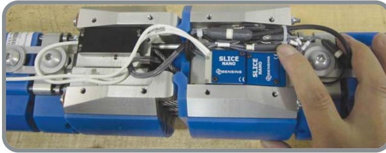
**12 channels of SLICE NANO™ installed in Flex leg:
