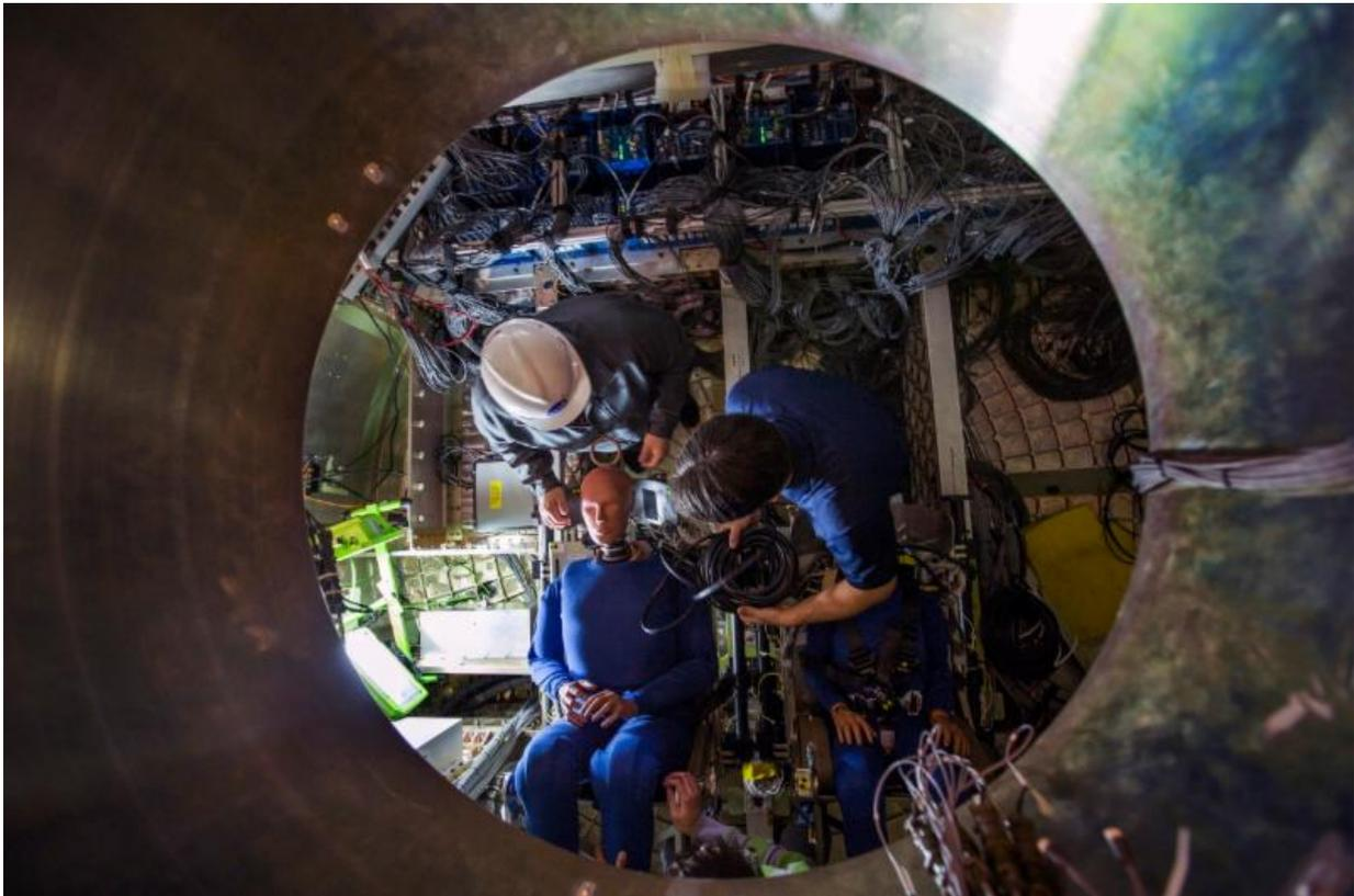
Inside the Orion test capsule, NASA engineers secure a male and female test dummy in the crew seats in efforts to help ensure the crew's safety on future deep-space missions. Over 500 channels of DTS data recorders are onboard to capture critical test data, including the splashdown impact astronauts could experience when landing in the Pacific Ocean. Photo credits: NASA/David C. Bowman
