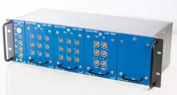
SLICE PRO LAB is a non-rugged, complete data acquisition system ideal for dummy calibration and static testing. The 19" rack includes an Ethernet Controller for start/status/power/comm and accommodates up to four SLICE PRO LAB modules (SIM, TOM or TDM). Compatible with both SLICEWare & DataPRO software.
