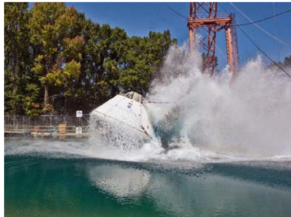
DTS TDAS systems on-board capture Orion splashdown data at the Langley Research Center test pool.
