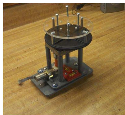
First generation rate table built by CSULA students with an electronics budget of $10
