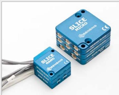
YES, but due to the harsh nature of many dynamic test sequences, DTS recommends following good grounding and shielding practices to maximize protection and keep systems functioning properly. Ground all DAS equipment, power supplies and sensor mounting fixtures whenever possible. Ground all SLICE enclosures to the test article.
