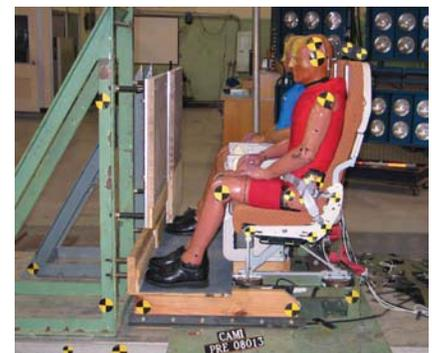
DTS customers including Wright Patterson AFB (top) and the Federal Aviation Administration (FAA) (bottom) use DTS data acquisition systems to perform a variety of regulation safety tests. Testing on passenger and crew seating, safety restraints and ejection seats have all aided in the trend of improved safety statistics.
