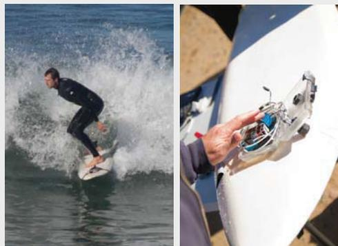
**Recently, a SLICE NANO miniature data recorder was used to capture surfboard dynamics in a real-world environment. The goal is to be able to collect and analyze enough data to be able to match the perfect surfboard and rider for every type of surf condition.**
