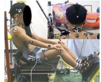
DTS ARS sensors and a TDAS data acquisition system were used to record the responses of an anthropomorphic test device (ATD) and human volunteers. Comparing & evaluating the test results will help improve safety devices with the goal of reducing injuries sustained by children, especially in car accidents.
