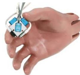
Both blocks include mounting holes for Endevco and MSI sensors to create a custom 6-degrees-of-freedom sensor package.
