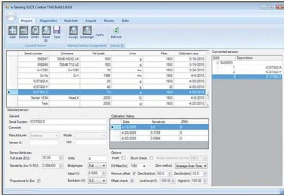
SLICEWare's sensor database allows for easy management of large or small sensor inventories. The integrated view of available SLICE systems makes sensor assignment with electronic ID or manually a snap.
