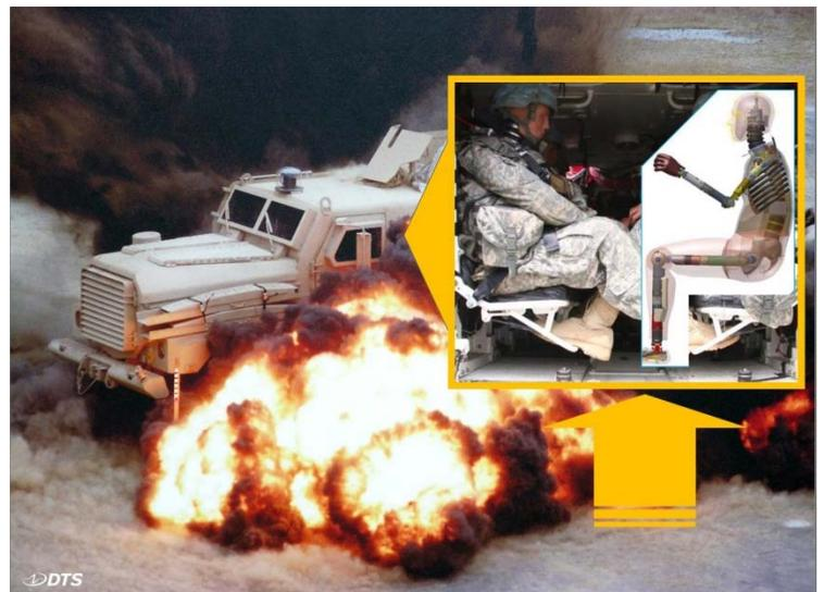
DTS has been awarded a contract by the U.S. Army to develop the first military blast test dummy, plus a new high-tech data recorder that fits inside to help assess potential skeletal injuries of soldiers exposed to under-body blast events like those from improvised explosive devices.
