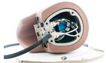
Moving the data recorders and sensors inside the test dummy heads eliminates big bundles of cables that can get tangled during testing.
