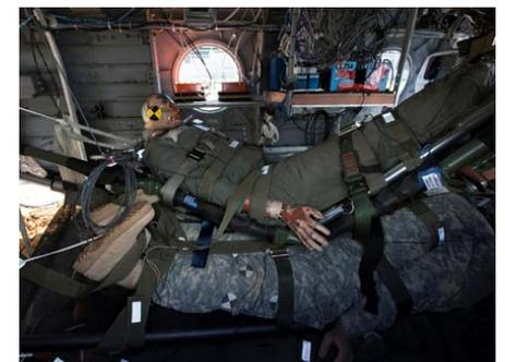
*Crash test manikins designed to measure human injury and survivability were equipped with sensors and DTS TDAS G5 data acquisition systems to record the valuable test data.*
