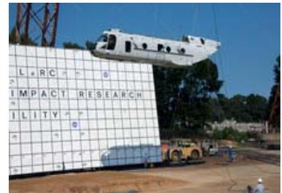
*Technicians at NASA Langley hoisted the 10,500 pound helicopter instrumented with data recorders and 15 test manikins 30 feet into the air before dropping it at 30 mph.*
