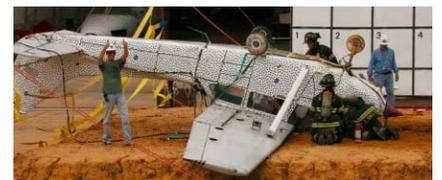
After being hoisted 100 feet in the air, the Cessna 172 hit the ground tail first and flipped over, simulating a severe, but survivable crash. NASA researchers will examine data captured by DTS data recorders to learn how crashes affect emergency locator transmitters.
