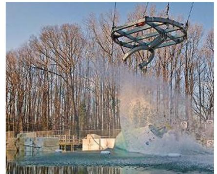
*In a series of splashdown tests at Langley Research Center, NASA dropped the 18,000 lb. Orion mockup capsule into a special test pool to re-create the splashdown anticipated for the Orion capsule's inaugural space mission Dec. 4, 2014. DTS data recorders and software were used on-board the capsule to capture important structural and crew safety test data.*
