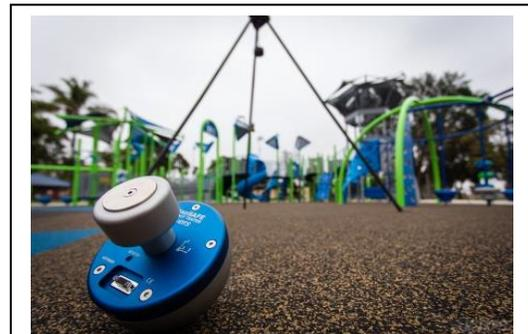
The cable-free HeadSAFE Impact Tester from DTS is a sphere that simulates a child's head and is used to evaluate the safety of recreational surfaces like playgrounds. A built-in data logger with XYZ accelerometers captures impact data to calculate head injury potential.
