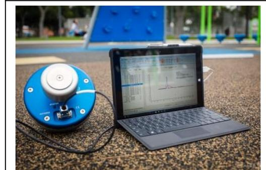
The ASTM/EN-compliant HeadSAFE stores up to 2,000 events in flash memory. Easy to use software lets field inspectors and surface manufacturers run custom reports on the spot.
