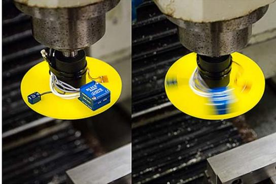
A 3-channel DTS SLICE data recorder, including battery, is mounted directly on a CNC shaft along with strain gauges to measure torque and a DTS ARS PRO angular rate sensor to measure angular velocity.
