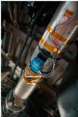
SLICE (3 to 24 channel) data recorders are autonomous and can be mounted directly on drive shafts, rotors and even in track vehicle treads, eliminating the need for slip rings or telemetry for measurements on rotating devices.
