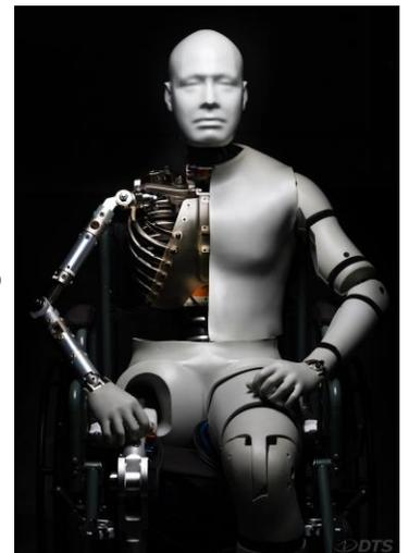
"The program provides a state-of-art test capability to assess potential skeletal injuries of Soldiers exposed to under-body blast," said Fred Hughes, director of the WIAMan Engineering Office. "The manikin's sophisticated biofidelity and robust sensor design provides an unmatched level of accuracy determining the potential effects of blast on Soldiers in new vehicle systems. The WIAMan effort is an example of outstanding collaboration among academia, industry, and the government."
