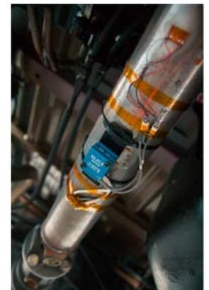
SLICE can be mounted directly on drive shafts, rotors, wheel hubs and other test articles or integrated into test dummies and head and leg forms.
