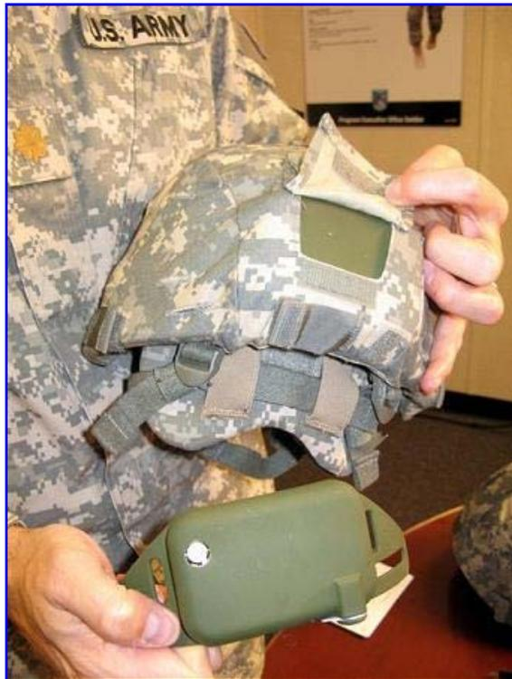
*The U.S. Army's Program Executive Office Soldier pushed the concept of a helmet-mounted sensor able to collect blast data from concept to fielding in a record six months. The 101st Airborne Division is receiving the sensors before its deployment to Afghanistan. Photo by Donna Miles*
