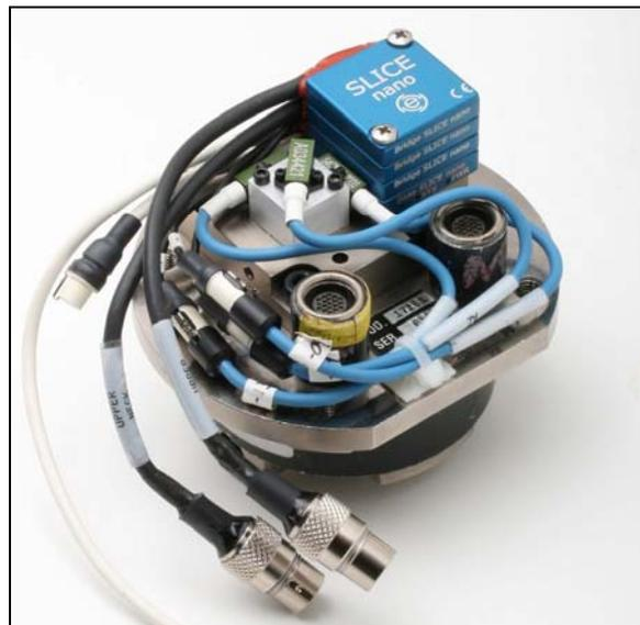
***Nine-channel SLICE NANO™ mounted on Hybrid III 6 year old upper neck load cell.***
