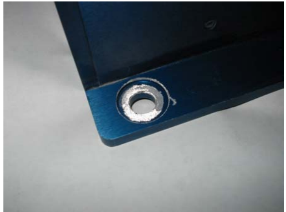
An adequately prepared mounting area (TDAS PRO rack cleaned to produce a grounding area)
