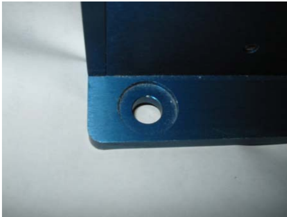
A poorly prepared mounting area (older style TDAS PRO rack)
