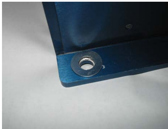
The preferred method for mounting area preparation (all new TDAS PRO racks are shipped with no anodizing under the washer to produce the best grounding area)
