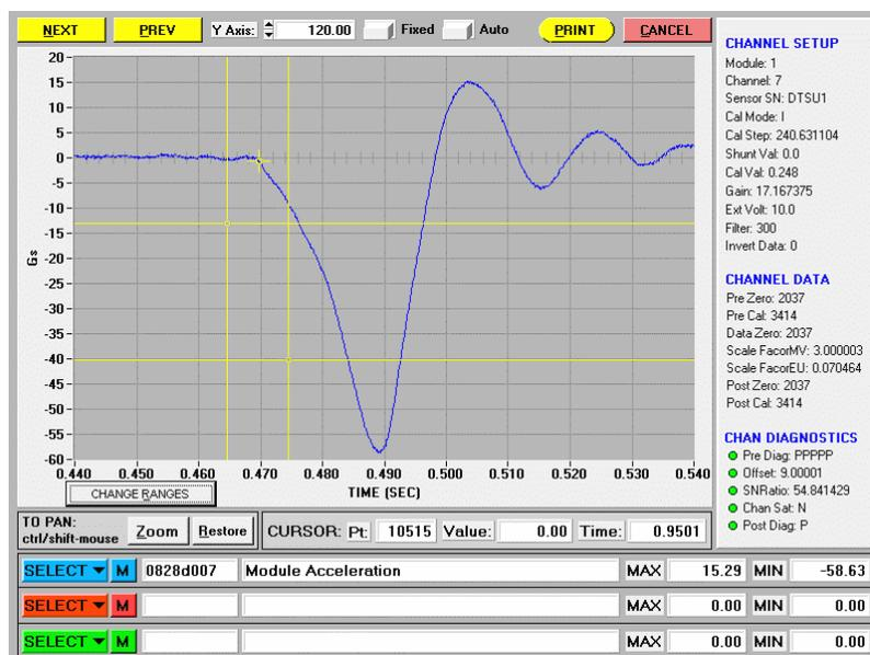
Figure 3: Durability test acceleration pulse.
