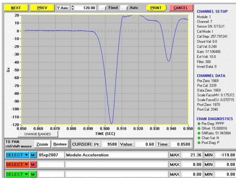
Figure 2: Standard production test acceleration pulse.
