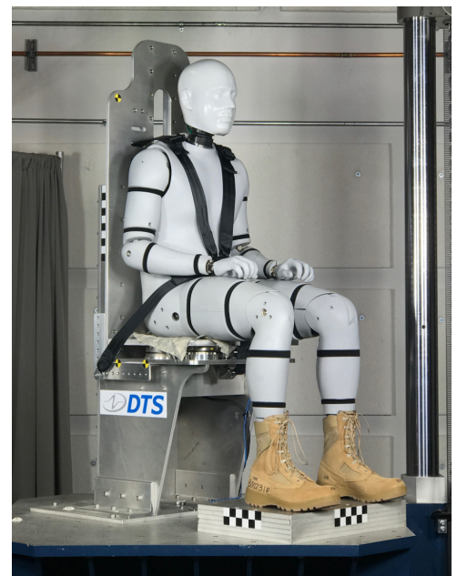
WIAMan with 146 SLICE6 HB channels
